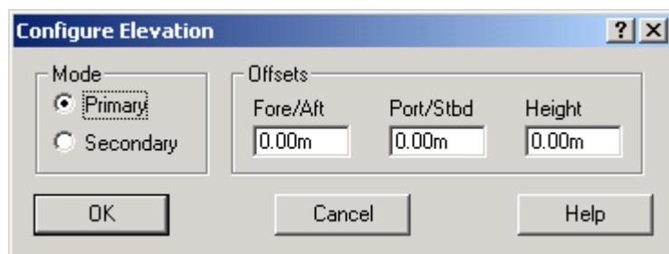
On this dialog you can specify if the PVP II D&H device is to be used for measuring the depth, as well as recording depth data in the raw files, by selecting the device as Primary. If Secondary is selected, then the depth measured from the device will be recorded in the raw files but will not be used for real time depth measurement.
